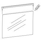
Remove the protective film and apply a thin line of glue to the top edge of the pane. Slide the molding into position. Be sure it is centered before the glue sets.
